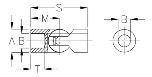
$\begin{array}{lll} A & = 28 \\ B \ H7 & = 14 \\ M & = 35.0 \\ Max \ torque \ (Nm) = 50 \\ s & = 70 \\ T & = 17 \end{array}$
